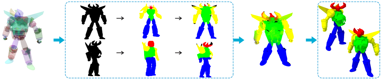
(b) Robot (1696 pieces, 76227 triangles): In the bottom projection, the wings of the input robot are incorrectly labeled as arm (yellow color), whereas an arm is incorrectly labeled as body (green) and leg (blue). However, the final labeling result is correct.
