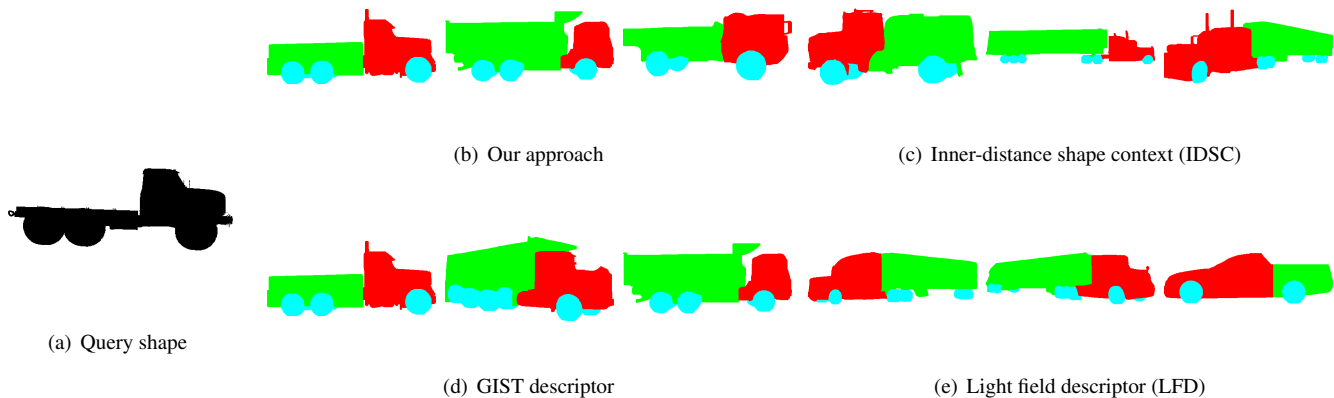
Figure 4: Visual comparison for shapes retrieved by different approaches for a truck projection (a). Our approach (b) returns shapes that have similar overall topology and similar views as the projection. Some of the shapes retrieved by existing approaches have incorrect views.
